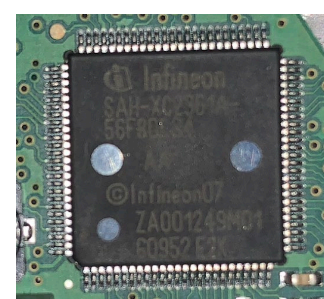
Figure 4. Closeup of an ACM microcontroller containing EEPROM: 512 Kbytes of flash memory.
