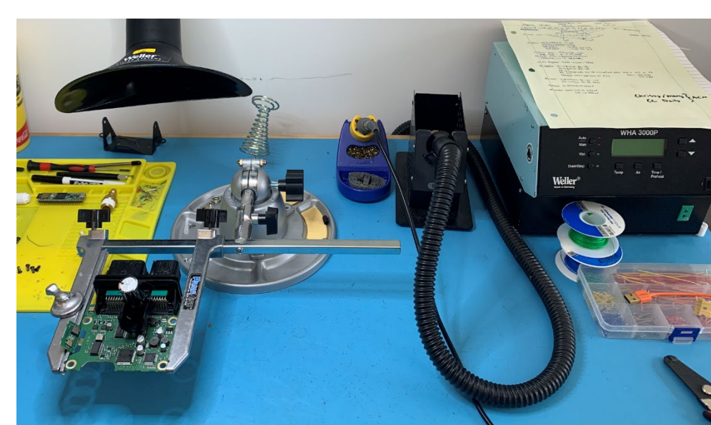
Figure 5. Workstation set up with heat gun, solder iron, tools, and ACM chip being transferred.
