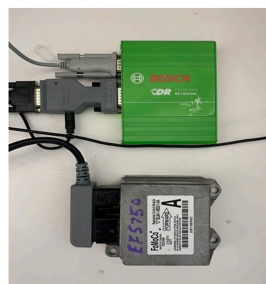
Figure 1. BOSCH Crash Data Retrieval (CDR) tool connected to an ACM for extraction.
