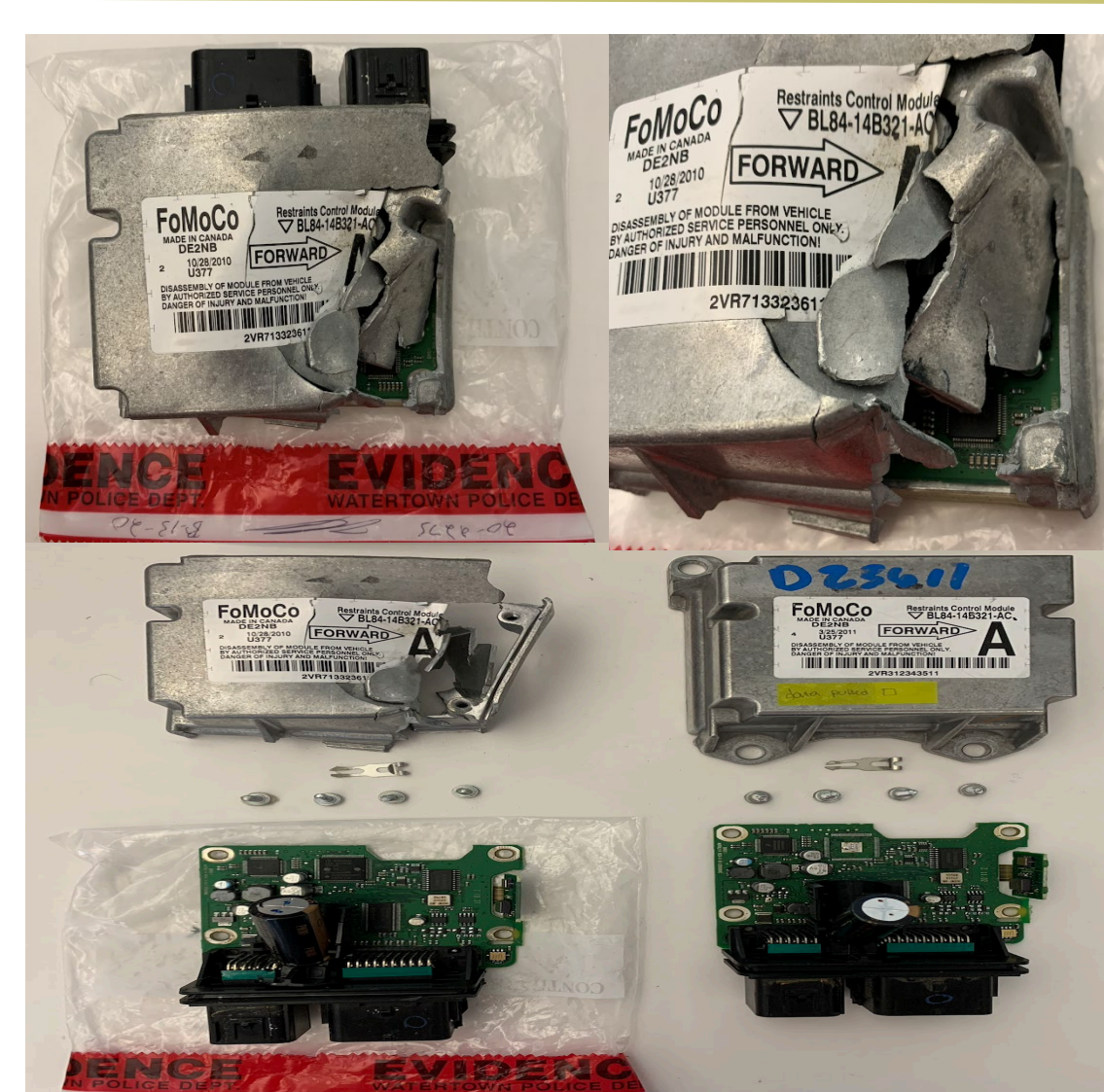
Figure 2. Images of an ACM that have been damaged from a crash.
